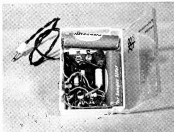
The transistor amplifier can be easily built into a small plastic box.
